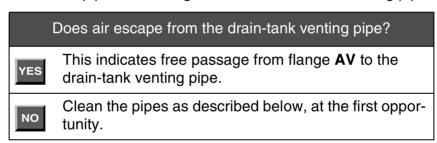
4. Check the pipes from the test-cocks to flange **AV**:
