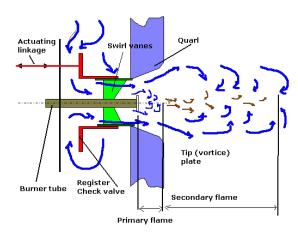
Another important factor for the formation of the primary flame is that it must be supplied with primary air in the correct proportion and at the right velocity. In the case of air registers using high velocity air streams this is done by fitting a tip plate that spills the primary air over into a series of vortices. This ensures good mixing of the air and fuel and, by reducing the forward speeds involved, helps to maintain the primary flame within the refractory quarl.
